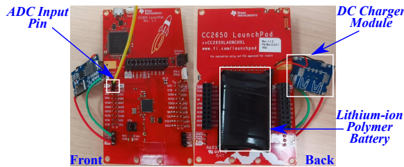
Fig. 1. The measurement device consists of a TI CC2650 Launchpad, a DC charger module, and a lithium-ion battery.
