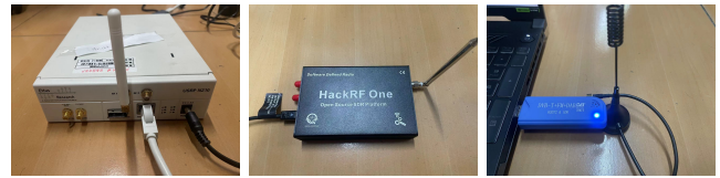
(a) USRP N210 as transmitter. (b) HackRF One as receiver. (c) RTL Dongle as receiver.
