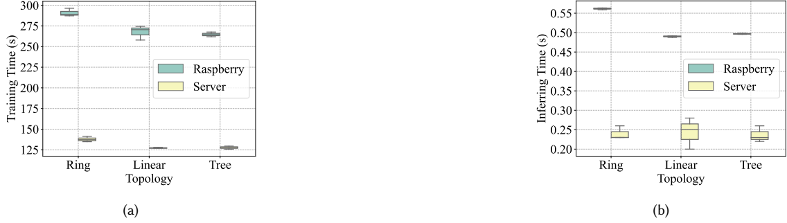
Fig. 15. (a) The training time comparison and (b) the inferring time comparison of DiRTS on Raspberry Pi and a server. In (a), the three bars below 150s are all tested on Server. In (b), the three bars above 0.45s are all tested on Raspberry Pi.
